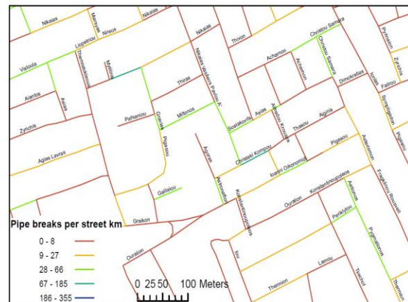
Figure 3. A chloropleth map illustrating the number of pipe breaks per street segment kilometer, in streets of Limassol during the year 2010. A natural junks classification with 5 categories is used for the illustration.
