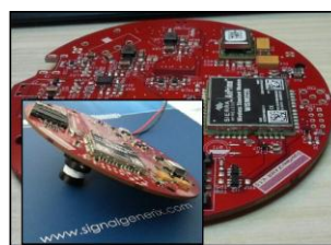
Snapshots of the developed PCB for automatic meter reading (AMR)
